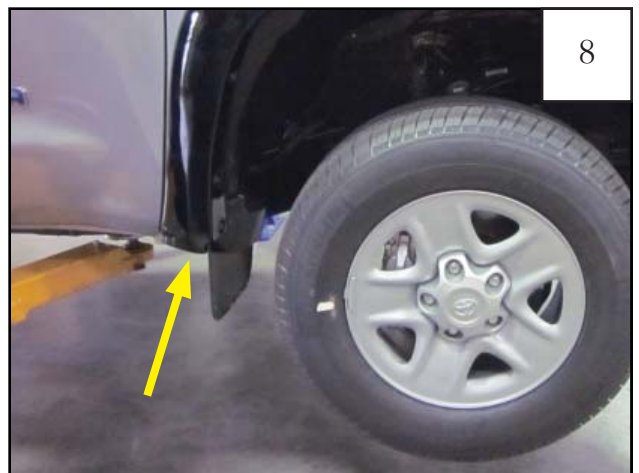
Install supplied push retainer (RV1-P009) into factory hole on underside of mudguard.
