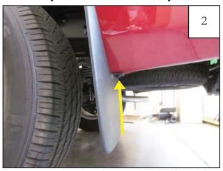
Remove one hex bolt from underside of mud flap using a 10mm socket. Discard mud flap.
