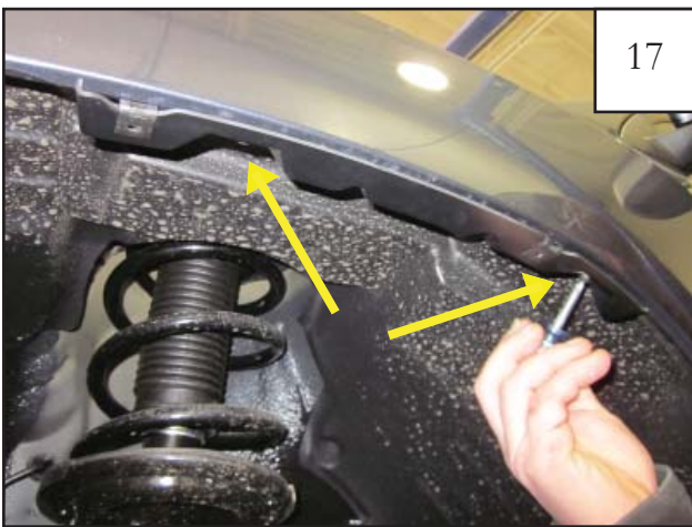
Hold front flare inner piece in wheel well with angled hole locations aligned with clips installed on wheel well lip in Step 12. Using a #2 Phillips Screwdriver, install Screws (SW1-0058) through front flare inner piece, through wheel well liner, and into Clip. Make sure that the corners of the Front Inner Piece are mounted flush with the sheet metal.
