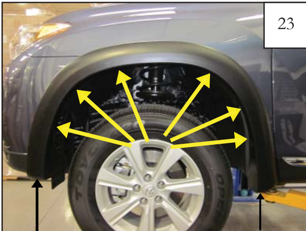
Once all hardware is started, check flare for proper positioning. Apply pressure at each fastening point and tighten all screws and bolts.
