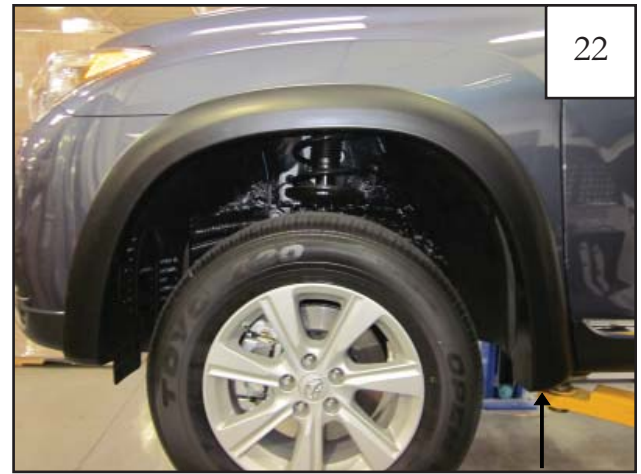
Install a Tuflock (RV1-P001) through flare and into sheet metal of wheel well where rear and lowermost plastic factory fastener was removed in Step 7.
