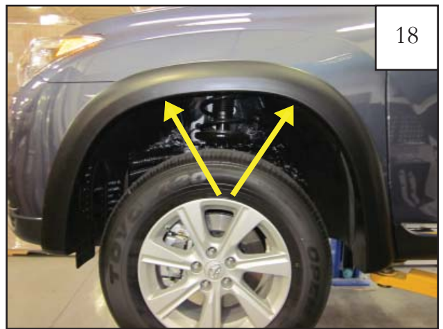
Hold flare to vehicle. Start Screws (SW1-0058) through two uppermost locations with #2 Phillips Screwdriver. Do not tighten.
