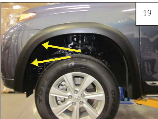
Using a #2 Phillips Screwdriver, install Screws (SW1-0057) through two frontward locations inside wheel well. Do not tighten.
