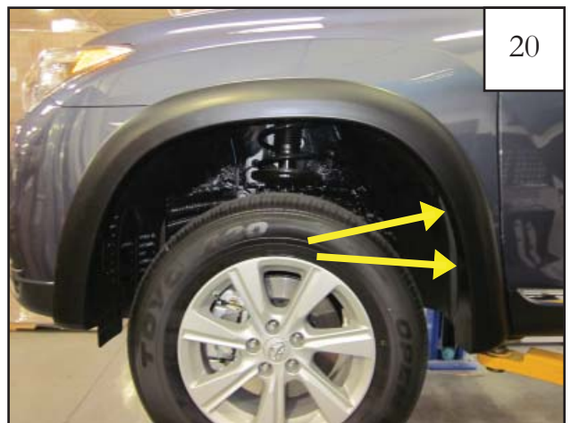
Start factory screws removed in Step 5 using a 3mm Allen Wrench. Do not tighten.
