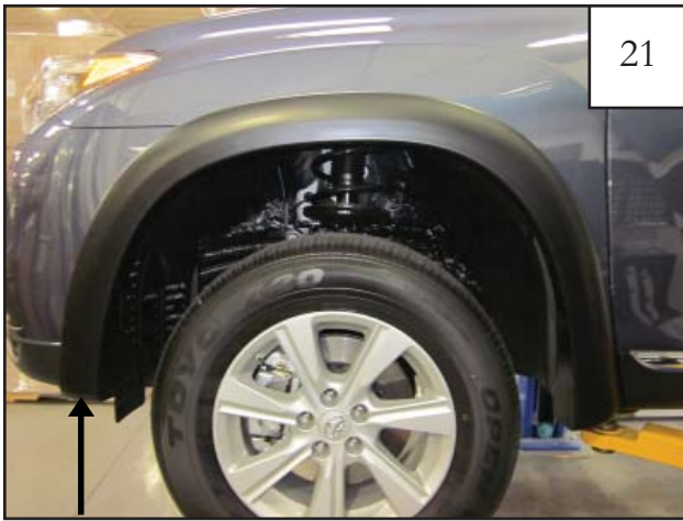
Using a 10 mm socket wrench, reinstall factory bolt removed in Step 1 by threading through flare.
