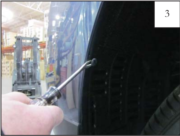
Using a pry tool, remove two plastic factory fasteners.
