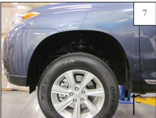
Using a pry tool, remove plastic factory fastener at lower rear of wheel well.
