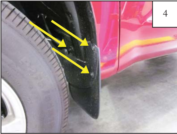
Remove three hex bolts from factory mud flap, using a 10mm socket.
