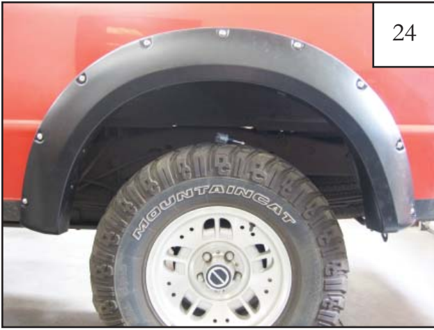
Completed rear flare installation.
