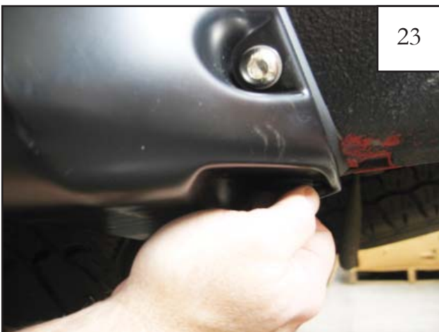
Start Fender Brace Nut removed in Step 17 on fender brace bolt.
