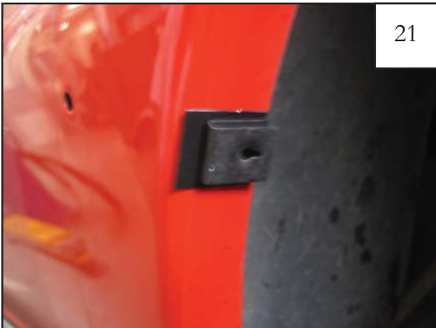
Install an Clip (CL1-0005) over each of the Tabs installed in Step 20.
