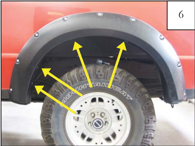
Mark through all flare holes using a grease pencil. Remove Flare.
