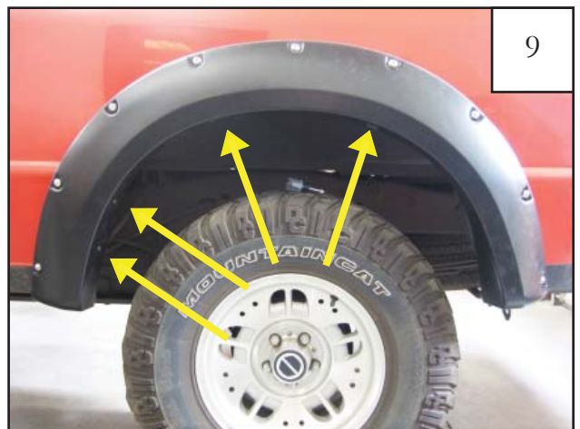
Reposition flare on fender ensuring that fender brace bolt is through lowest rearward hole and, starting with the rearmost wheel well hole, start Screws (SW1-0050) through holes in flare and into Clips (CL1-0022) with a #2 Phillips screwdriver.
