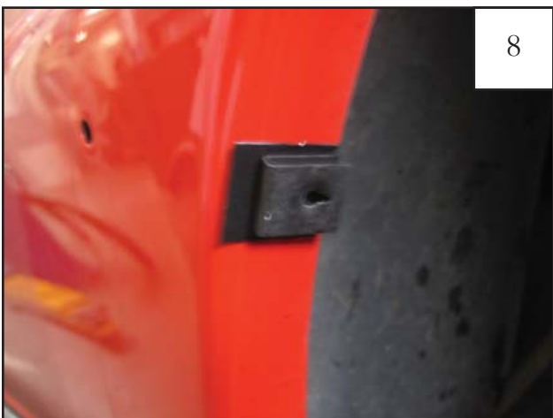
Install an Clip (CL1-0005) over each of the Tabs installed in Step 7.
