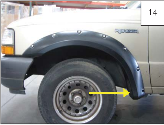
Reinstall factory screw saved from Step 8.
