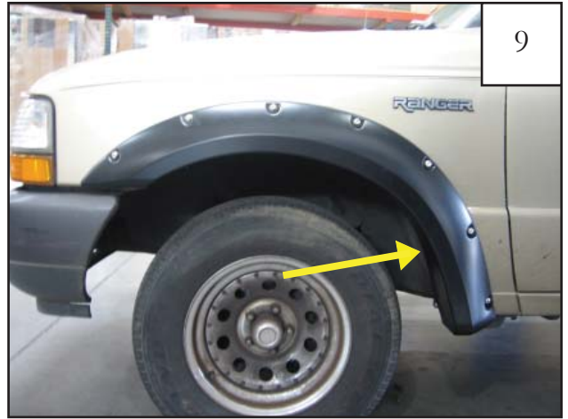
Hold flare to vehicle and mark second rearmost hole location with grease pencil.
