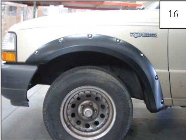
Completed front flare installation.
