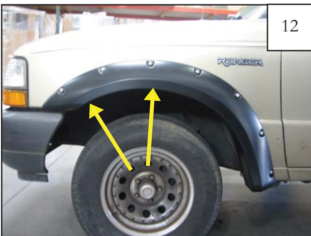
Hold flare in place and start Screws (SW1-0058) in Clip (CL1-0022) locations and into inner piece. Do not tighten.
