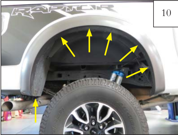
Using a pry tool, remove 5 retainers from the factory flare. Discard factory retainers.
