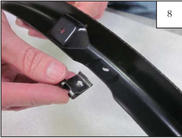
Attach 3 "U" clips (CL1-0022) to the inner bracket as shown.
