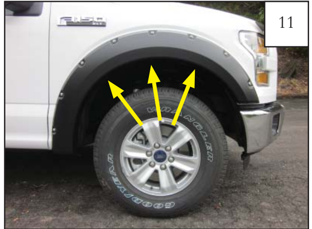
Position flare on fender, pressing inward on the flare, line up the flare mounting holes with the mounting clips on the inner piece. Install 3 Phillips Truss Screws (SW1-0058) through the flare and into the clips on the inner piece. Do not tighten. (3 locations)
