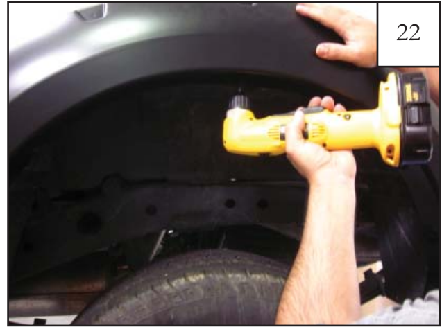
While using an electric drill install one (1) supplied self tapping screw (SW1-0066) into the center top location of flare and into sheet metal using hole in flare as a guide.
