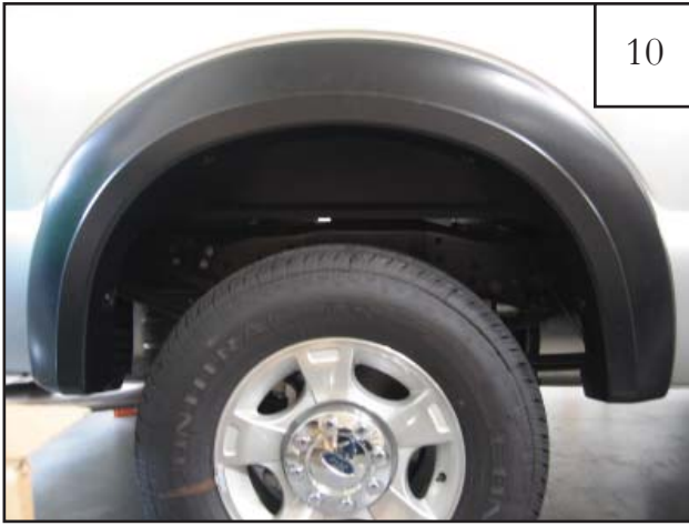
Completed rear flare installation.
