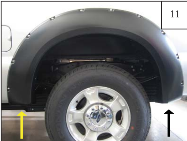
Using a 5/32" Allen Wrench and 3/8" socket, install bolt, Washer (WA1-0010), Spacer (SP1-0008), Washer (WA1-0017), and Nut (NU1-0015) through bottom two holes in flare and into factory holes. See step 12.
