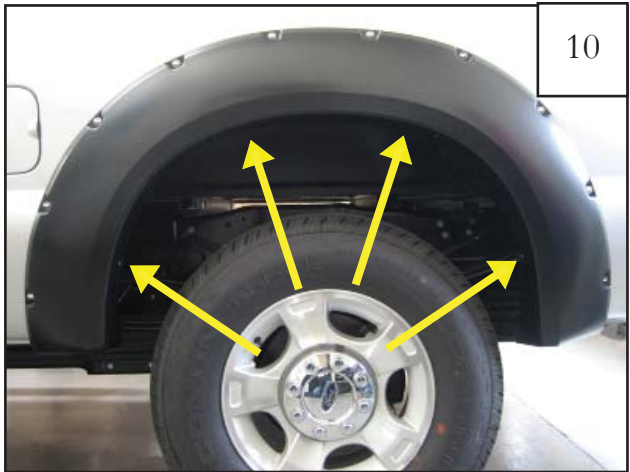
Position flare on fender and, starting with the two top holes, install Screw (SW1-0050)s through holes in flare and into clips with a #2 Phillips screwdriver.
