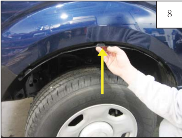
Using a Phillips screw driver, start a factory supplied screw through center hole in inner piece and through the speed clip over the fender wheel well lip.
