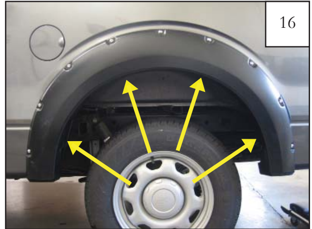
Hold flare to vehicle and mark the location with a grease pencil of the four holes in the flare.
