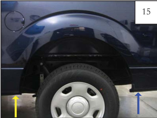
Remove two factory bolts with a 10 mm socket wrench. Save for reinstallation.
