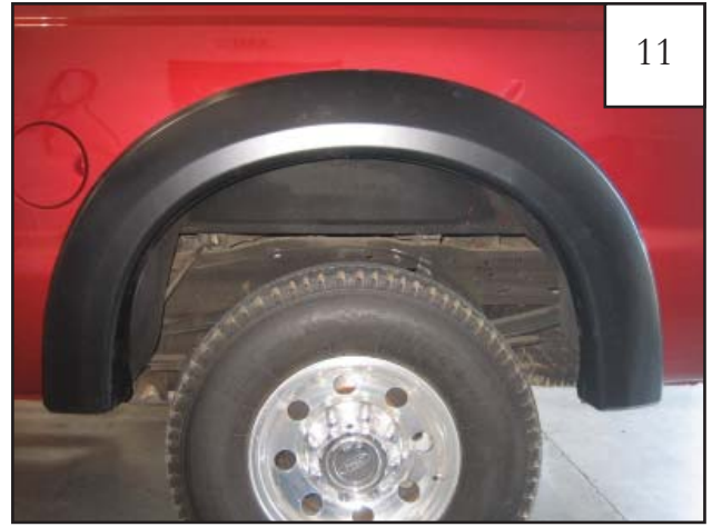
Completed rear flare installation.
