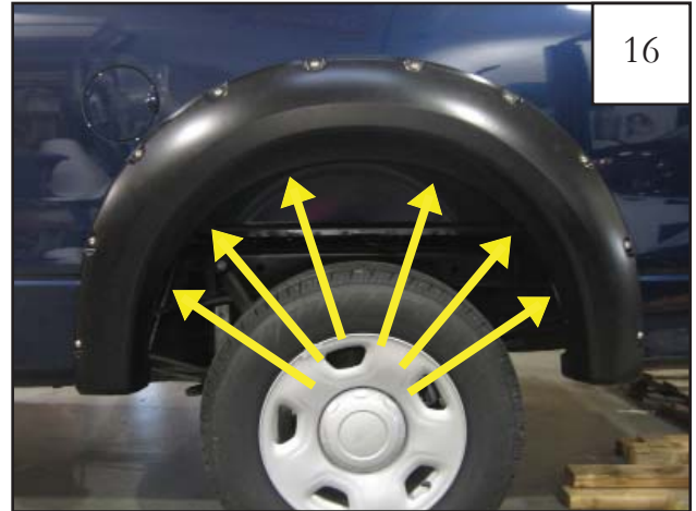
Hold flare to vehicle and mark the location with a grease pencil of the six holes in the flare.
