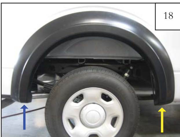
18 Using a 10 mm socket wrench, tighten 35 mm bolt through spacer and factory hole in sheet metal.
