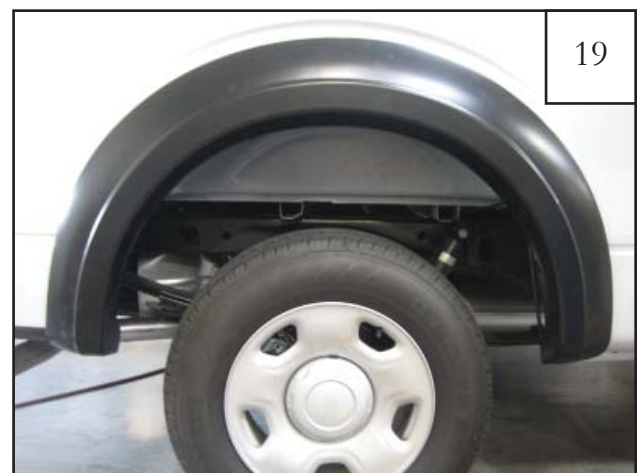
19 Completed rear flare installation.
