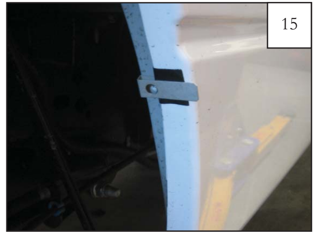
15 Install a long clip over each of the four black tabs placed on the sheet metal in Step 14.
