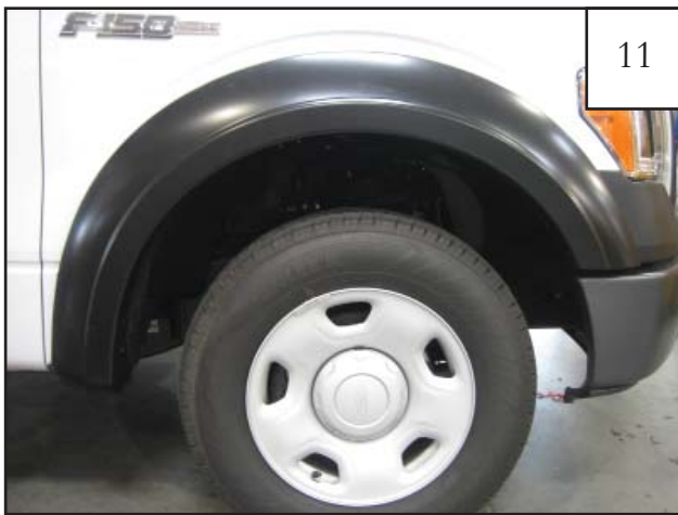
Completed front flare installation.
