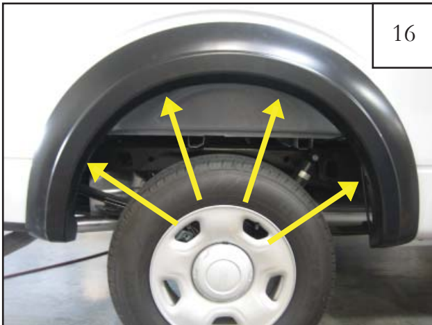
16 Hold flare to vehicle and start truss head screws through the two topmost holes in wheel well. Then start truss head screws through remaining two holes in flare. Tighten all screws.
