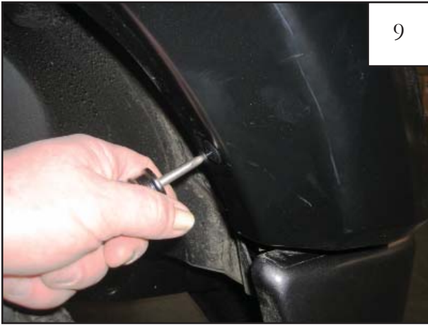
Still holding flare to fender, install tuflocks using a Phillips screw driver. See step 10.
