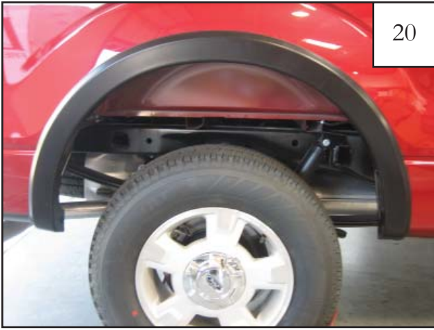
Completed rear flare installation.
