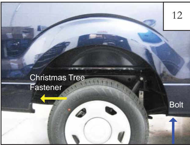
Remove one factory bolt from the forward, underside of the rear wheel well with a 10 mm socket wrench. Remove one Christmas tree fastener from the inside of the rearward inside of the rear wheel well with a trim tool.
