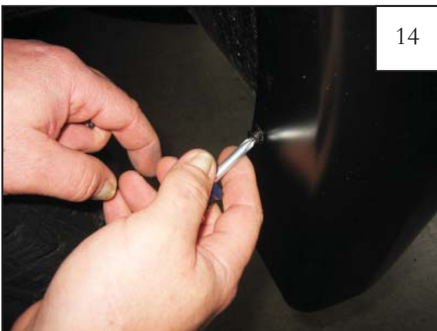
Install four supplied Screws (SW1-0050) through remaining holes and into clips installed in Step 12, working from front to back of wheel well.
