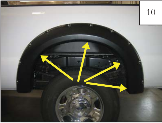
Clip locations. Use holes in flare to mark the four clip locations.
