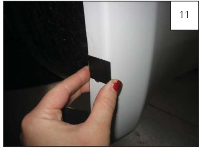
Remove flare and center a Tab (MT1-0002) over each of the four locations marked in Step 9.
