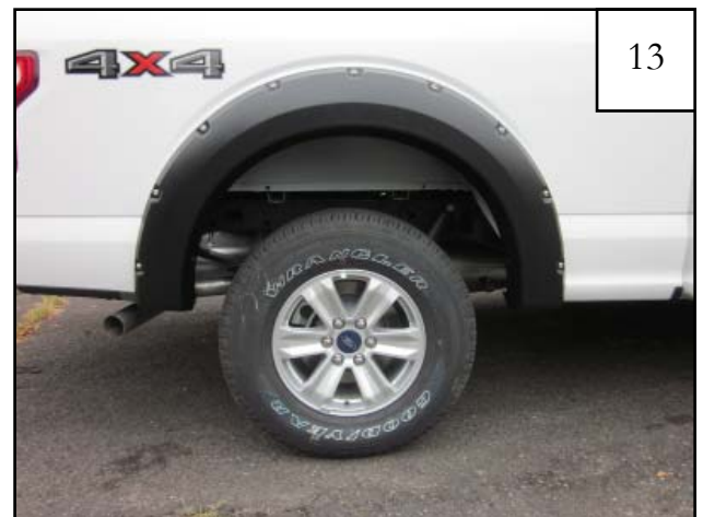
Completed rear flare installation.
