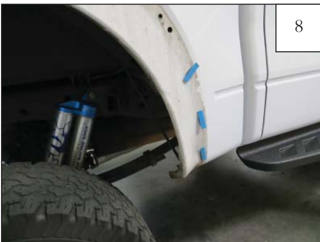
Using pliers, remove factory plastic clips. Clean the fender area.
