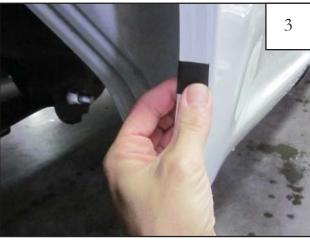
Wrap a Foam Tab (MT1-0034) around the wheel well sheet metal, centered over each of the upper four marks made in Step 2. Place a Mylar Tab (MT1-0014) at the mark made on the lower front of the wheel well.
