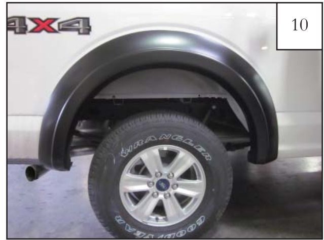
Completed rear flare installation.
