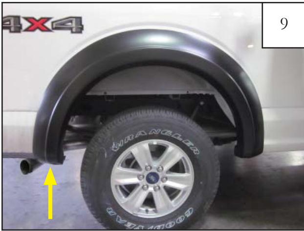
Install supplied push retainer (RV1-P0006) into flare and through factory hole at rear of wheel well.
