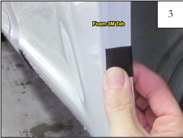
Wrap a Foam Tab (MT1-0034) around the wheel well sheet metal, centered over the mark made in Step 2.
