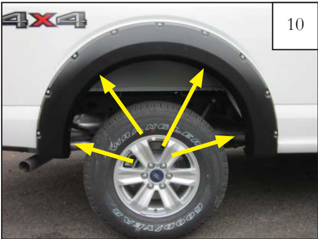
While holding flare to vehicle, start supplied screws (SW1-0058) through the four topmost mounting holes in flare and into the clips installed in Step 18.
