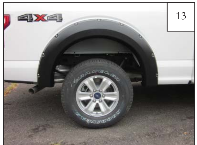
Completed rear flare installation.
