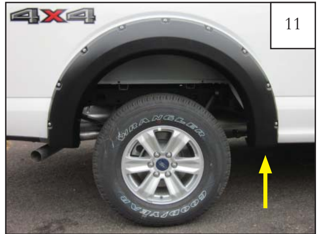
Start a supplied screw (SW1-0050) through the flare into the clip installed in Step 19. Tighten all screws.
