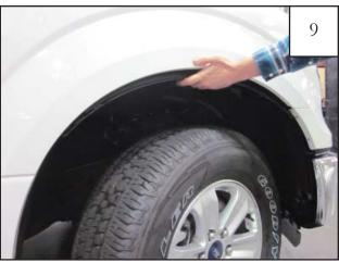
Line up the holes in the inner piece with the three uppermost factory holes. *NOTE: Driver's side inner piece is marked with an "LR" and passenger's side inner piece is marked with an "RR".*
