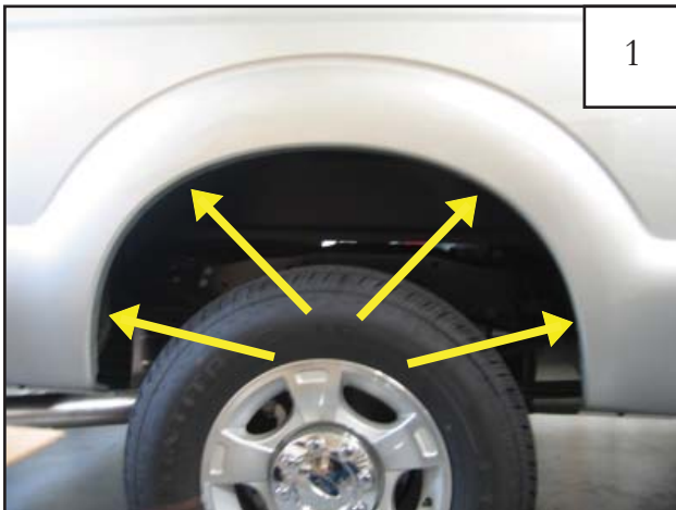
Hold flare to vehicle and ensure that four holes in flares line up with four factory holes in the fender.
