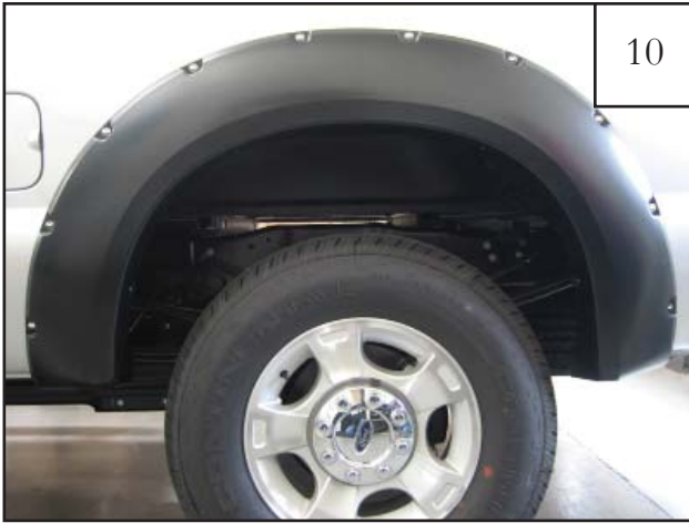
Completed rear flare installation.
