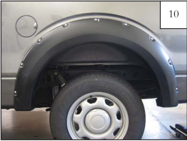
Completed rear flare installation.
