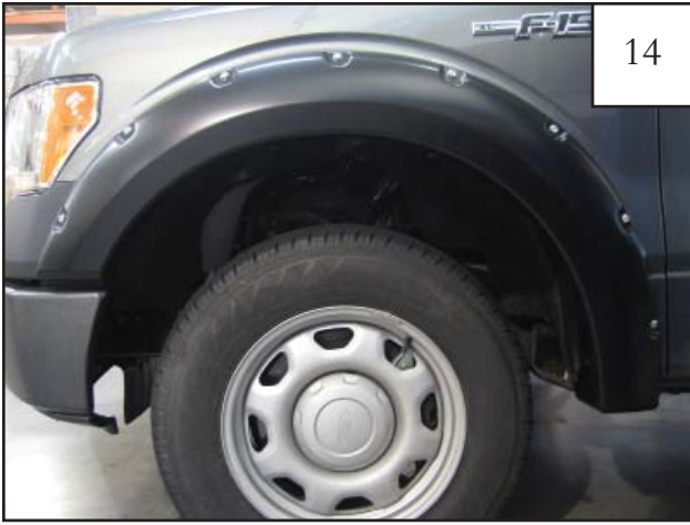
Completed front flare installation.
