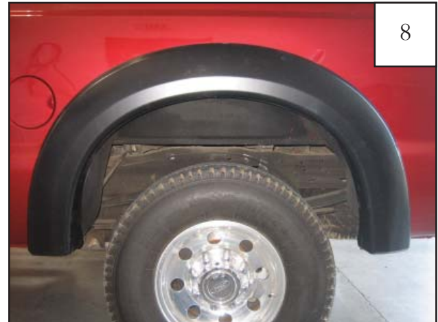
Completed rear flare installation.
