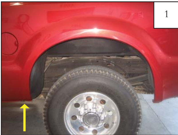
Remove one factory bolt with a 10 mm socket wrench, hold nut on bolt in place with a 13 mm wrench. Save bolt for reinstallation
