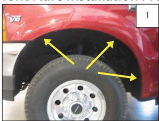
Remove three factory screws with a 7/32" socket wrench. Save screws for reinstallation.
