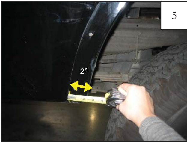
At FRONT of wheel well, use a tape measure and a grease pencil to mark a line 2" toward front of vehicle from fender lip (at bottom edge).
