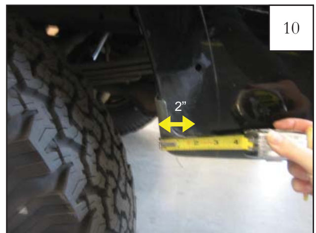
At REAR of wheel well, use a tape measure and a grease pencil to mark a line 2" toward rear of vehicle from fender lip (at bottom edge).
