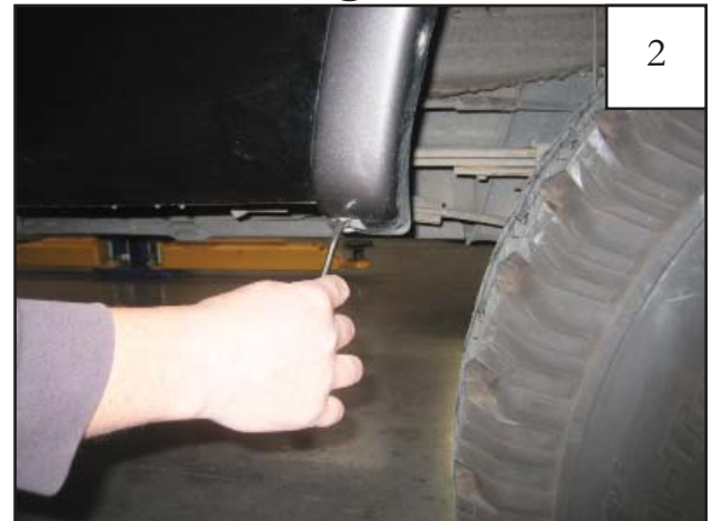
Use a trim tool to remove one plastic fastener located at bottom front of wheel well as shown.
