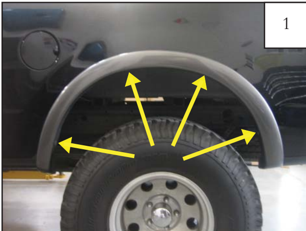
Using a #2 Phillips bit, remove four factory screws located inside wheel well (at locations shown).
