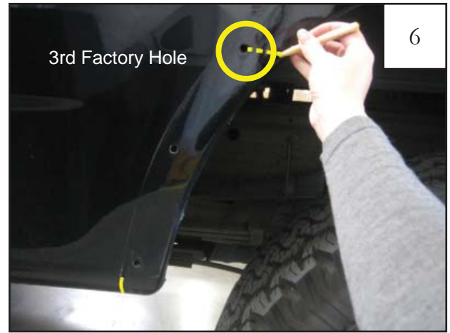
At fender lip, make a mark horizontal to the third factory hole up from bottom front of fender well.
