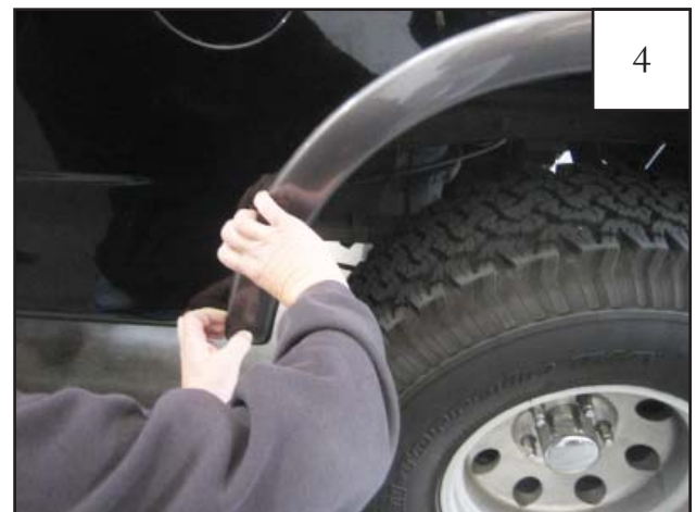
Starting at front of flare, pull firmly to release flare from fender, working your way to the back. You will hear popping noises as clips release. It is O.K. if clips break, they will be discarded.
