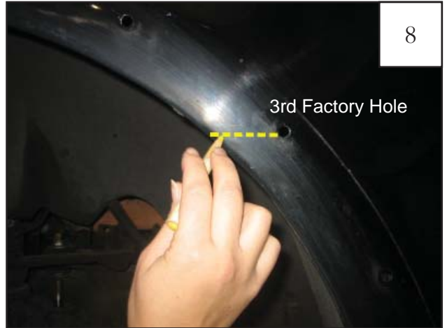
At fender lip, make a mark horizontal to the third factory hole up from bottom rear of fender well.
