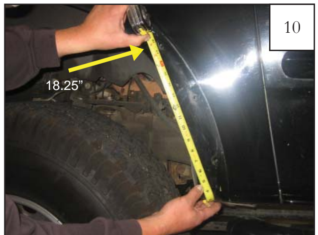
For trucks without factory flares ONLY: Wrapping tape measure up from bottom edge of sheet metal of inside of fender, measure up 21" and make a mark on fender lip where tape measure intersects.
