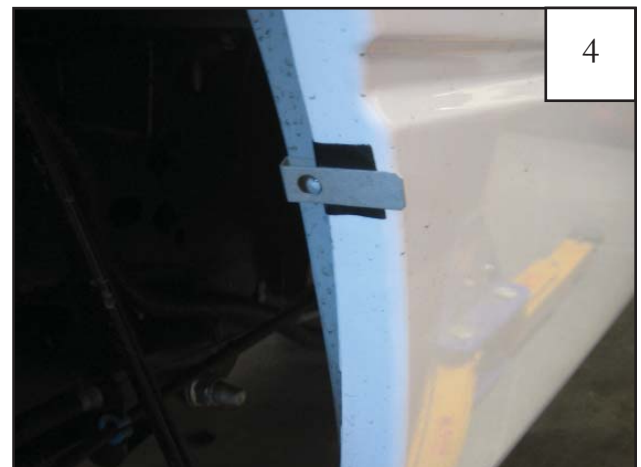
Install a long clip over each of the four black tabs placed on the sheet metal in Step 3.
