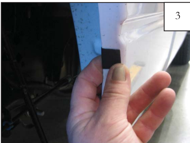
Wrap a black tab around the wheel well sheet metal, centered over each of the four marks made in Step 2.
