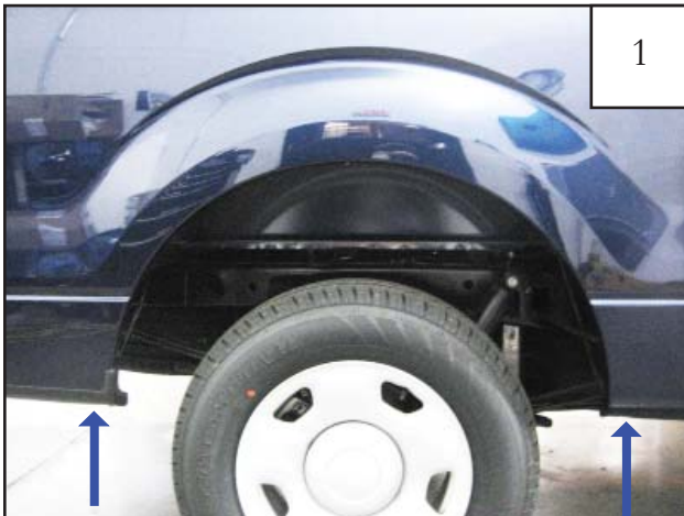
Remove two factory bolts with a 10 mm socket wrench.
