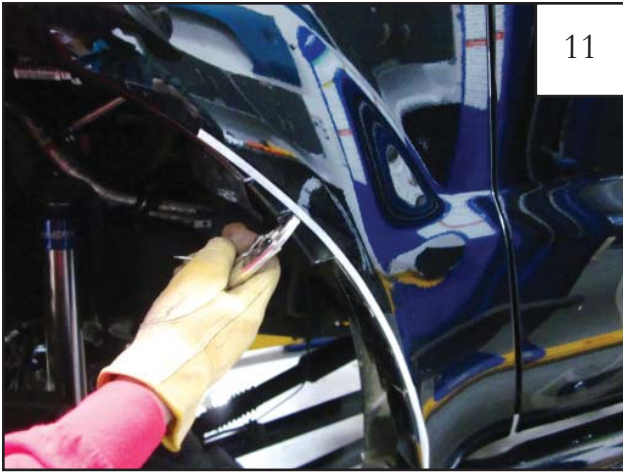
Bend tabs into wheel well with pliers and flatten.
