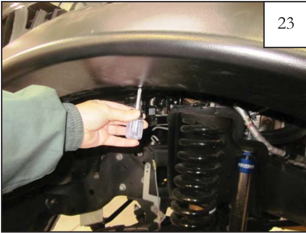
Install flare and start Screw (SW1-0056) through clips installed in previous step with a #2 Phillips Driver. Do not tighten.
