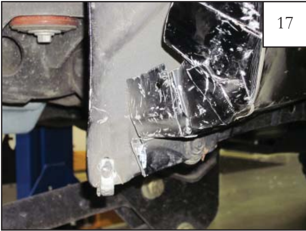
This is how it should look after you cut off back lower flange.
