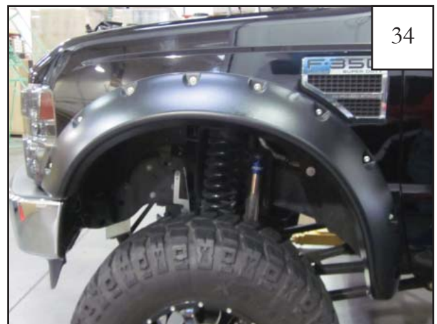
Completed front flare installation.
