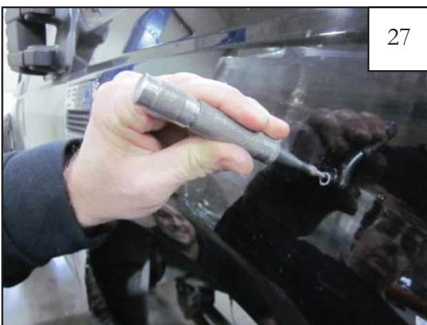
Remove screws and flare. Using marks made with scratch awl as a guide, use a center punch to score sheet metal prior to drilling.
