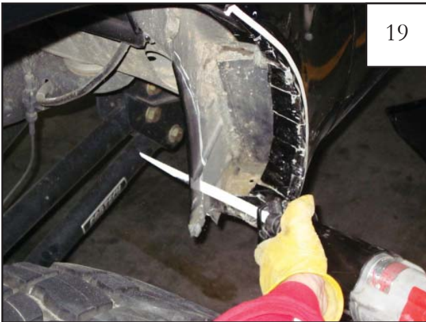
Using a Sawsall, cut along reference line.
