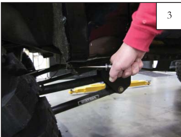
Using a pry tool, remove factory installed tufloc rivet located at the bottom rear of the wheel well.
