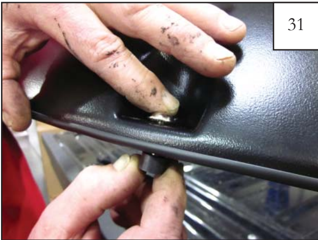
Thread bolt (SW1-0045) through pocket hole in flare then install spacer (SP1-0009) over end of bolt. Hand tighten spacer on bolt until snug near flare plastic.
