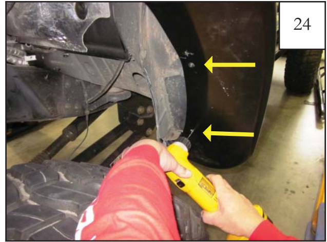
Hold flare tightly against fender, lining it up along style lines, drill into sheet metal through pre-drilled flare holes at rear side using 1/8" drill bit.
