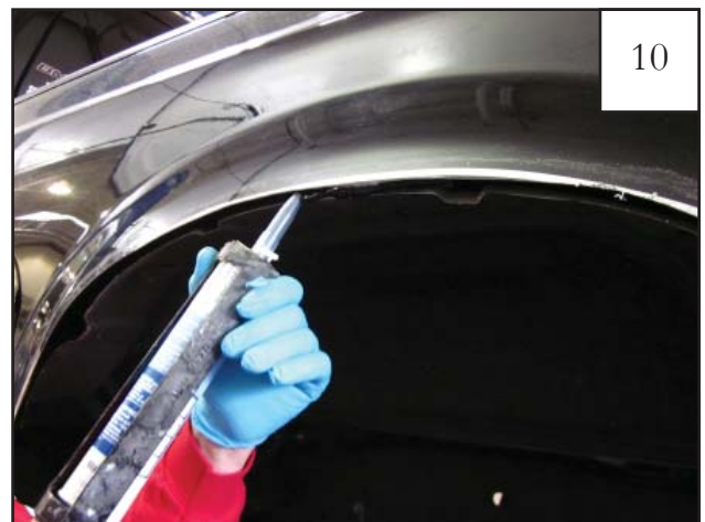
Use urethane caulking to fill between walls of cut fender. Follow caulk directions for drying time. See next step .
