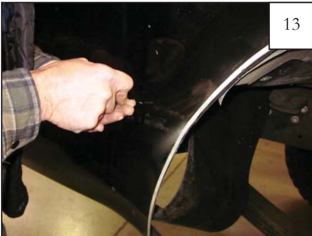
Using marks made with scratch awl as a guide, score the sheet metal with a center punch prior to drilling.
