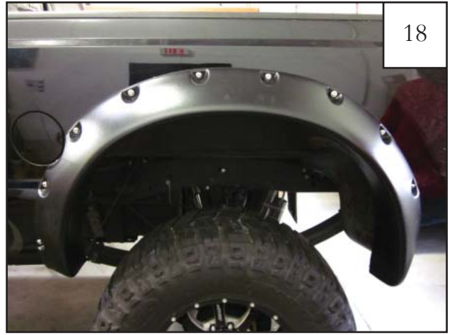
Completed rear flare installation.
