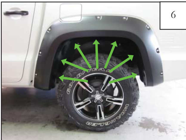
Using T-45 Torx bit, install 7 factory screws. Fully tighten all screws while pressing in on flare to ensure it is snug against sheet metal.
