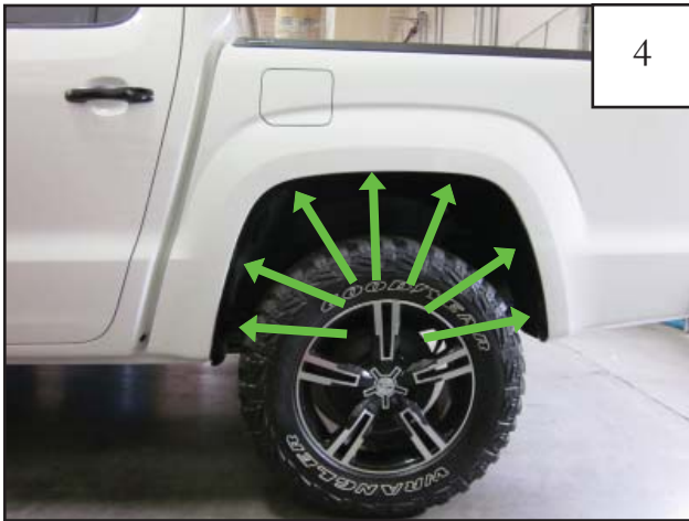
Using an T-25 Torx bit, remove 7 factory screws. Retain screws for reinstallation.
