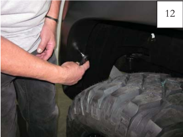
Reposition flare on fender. Using a #2 Phillips, start a supplied Screw (SW1-0058) through two forward hole locations and through each Clip installed in step 10. If needed, use scratch awl to locate holes.
