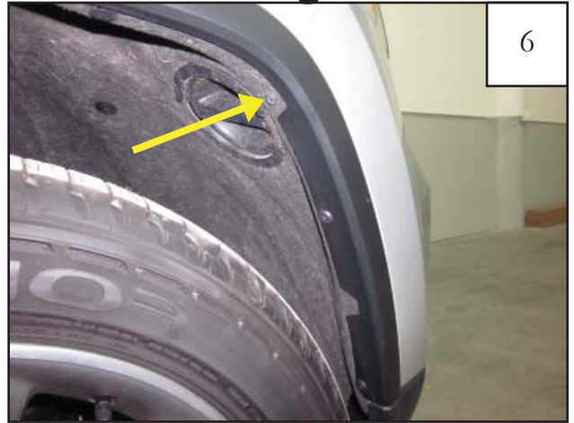
Using a 10mm socket and wrench, remove factory screw at indicated location in image above. Retain screw for reinstallation.
