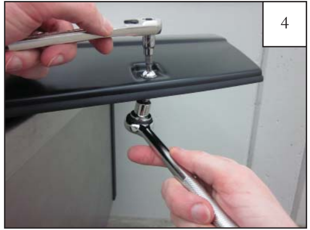
Fully tighten using an 8mm wrench or 3/8 ratchet with a 8mm socket for the Nyloc Nut, and use the supplied Torx Bit (SW1-0052) and wrench for the Bolt. Repeat for remaining pockets.
