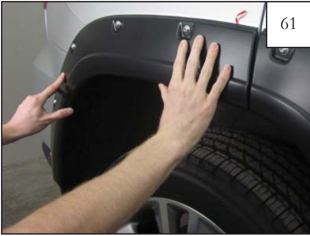
61 Hold Rear Main Flare up to wheel well to confirm fit. Do not install fasteners at this time.
