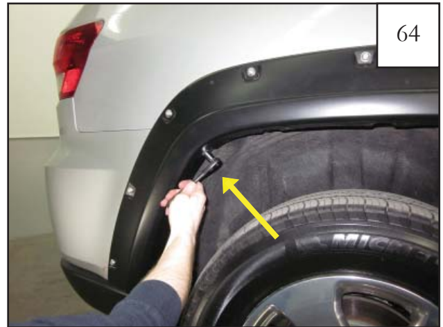
64 While holding Flare on vehicle, install factory fasteners removed in Step 31 & Step 57 using a 10mm socket and wrench. Do not fully tighten at this time.
