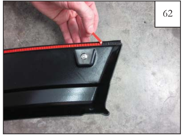
62 Pull back 1-2 inches of red tape liner from each end of installed edge trim and fold towards outside of the flare.
