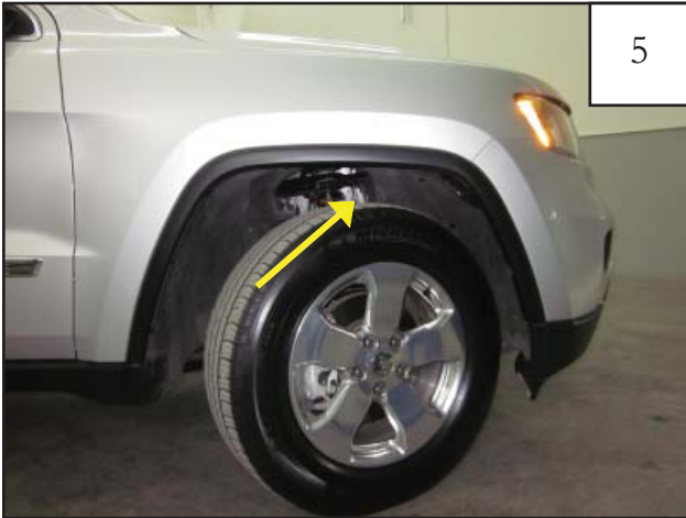
Turn wheel inward to give clear access to front of wheel well for installation.
