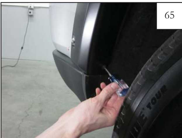
65 Using a Stubby or Right Angle Screwdriver, install supplied Screws (SW1-0056) thru flare and into clips installed in steps 58 & 59. Do not fully tighten at this time.
