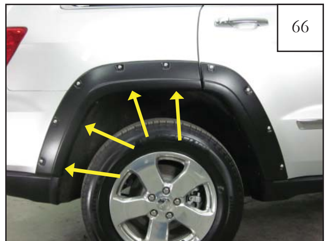
66 Screw/Clip locations (4 places). Ensure flare is properly aligned on vehicle. Style lines of Rear Door Flare and Rear Main Flare should match. Once properly aligned tighten all fasteners.
