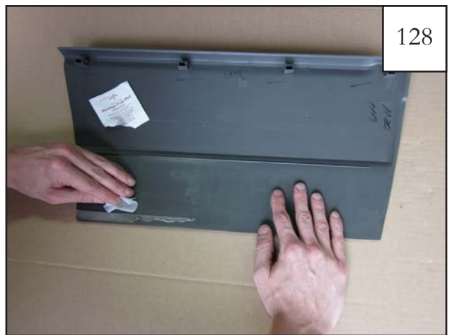
In preparation for applying new tape, use a supplied alcohol wipe (AD1-0010) to clean plastic and remove factory tape from side cladding.
