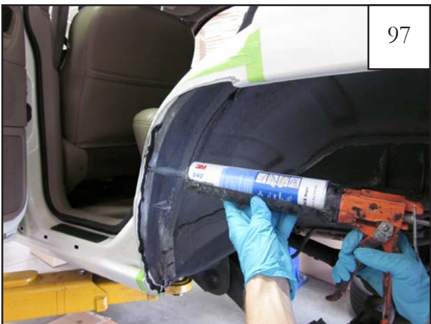
Apply urethane caulking or primer to all cut areas of wheel well to seal any exposed sheet metal for rust prevention.
