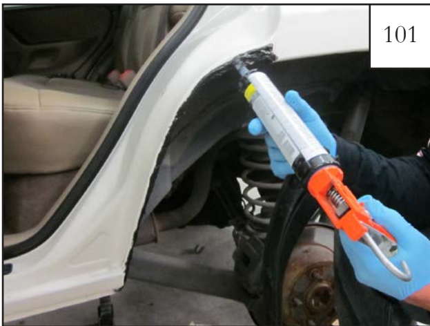
101 Prior to installation of the cut cover, apply another layer of caulking to help keep cut cover in place.
