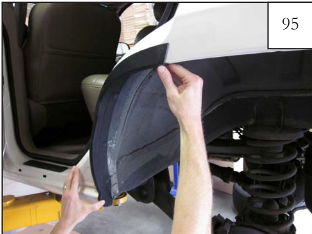
Hold cut cover piece in place on vehicle. Confirm fit to cut areas and make adjustments as needed. Parts are marked on the inside. Driver's side: D2 for cut cover piece.
