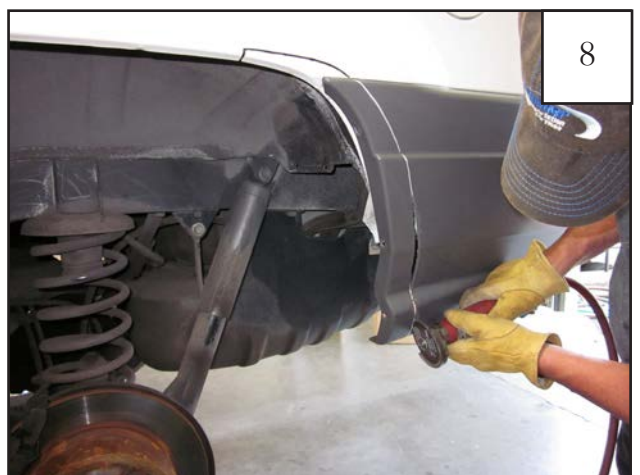
Using a cut off wheel, sawsall or other suitable tool, cut along line marked on bumper only. NOTE: DO NOT CUT SHEET METAL AT THIS TIME.
