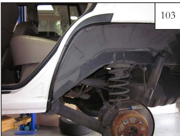
103 Installed cut cover.
