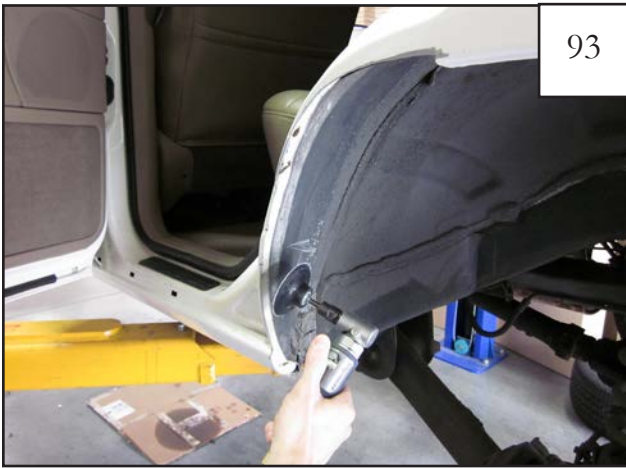
Using an angle grinder or sandpaper, sand and smooth cut along fender lip.
