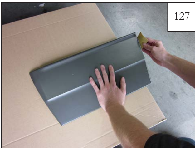
Using sand paper, smooth cut edge of the factory side cladding.
