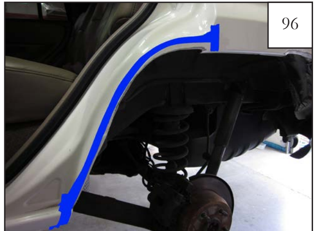
With door open, run masking tape along cut edges around door seam in preparation for sealing/caulking.
