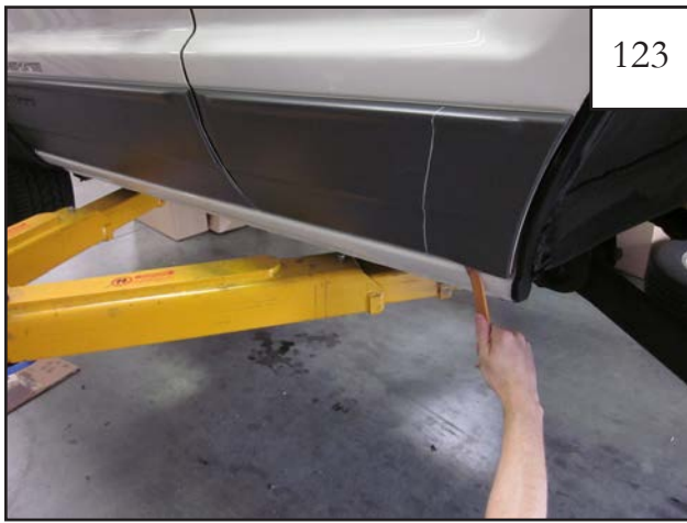
Using a pry tool, separate the factory side cladding from the sheet metal along the bottom taped edge.
