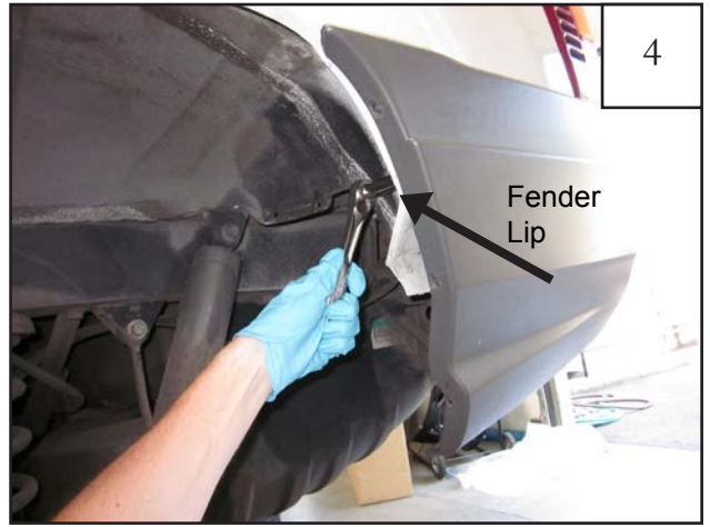
Using a 10mm deep socket and wrench, remove bolts on inner side of fender lip (2 locations).
