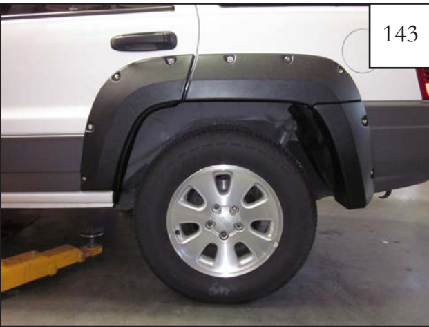
Completed rear flare installation.
