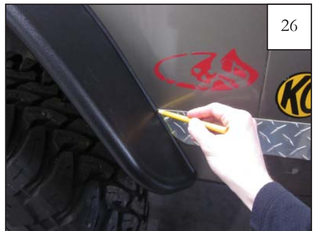
OPTIONAL: If aftermarket rocker pieces are installed, you may need to trim them for a proper fit. If so, place main flare over inner pieces and use a grease pencil to mark rocker pieces for trimming.
