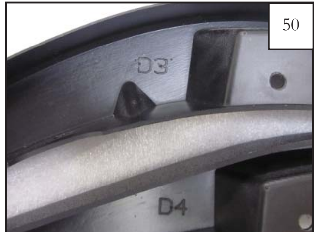
Locate the flat flare rear inner pieces. The driver side rear inner pieces are marked D3 & D4. The passenger side rear inner pieces are marked P3 & P4.
