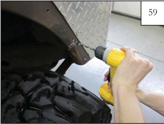
Using a 1/4" drill bit, drill marked hole.
