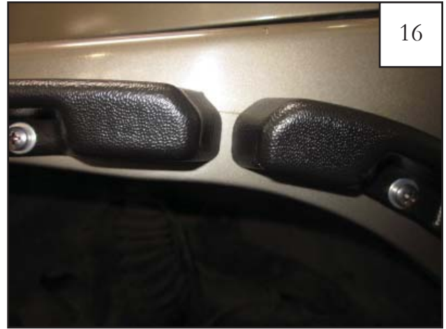
Make sure that inner piece D2 lines up with inner piece D1 before fully tightening. (for passenger side P1 and P2)
