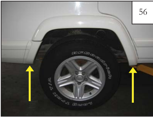
Remove the factory rear flare starting with the lowest factory fasteners. Use the following socket & wrench for factory fasteners: (84-96 Model Years = 7mm) (97-01 Model Years = 1/4")
