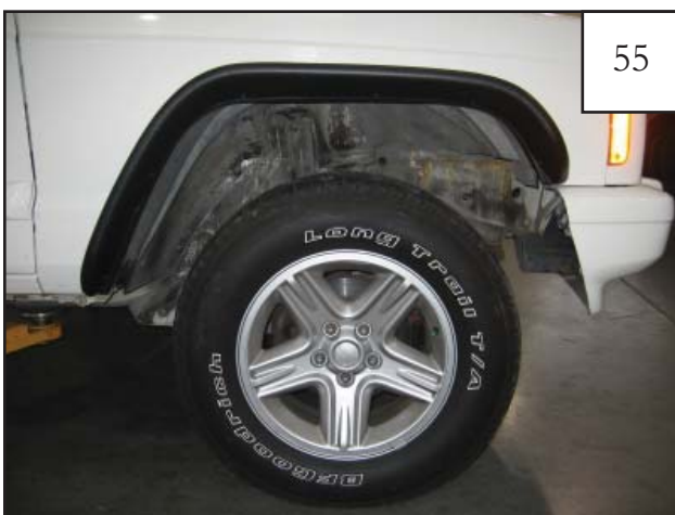
Completed front passenger's side flare installation.
