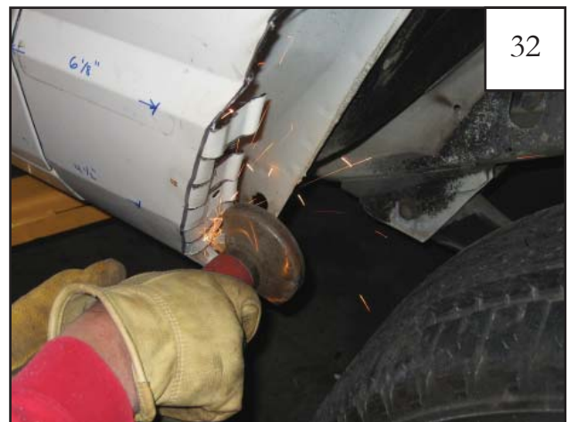
Use a cut off saw to cut exposed sheet metal where marked in previous step.
