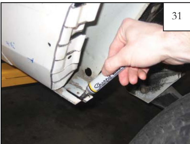
Mark cut lines on exposed sheet metal
