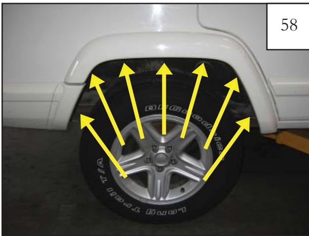
Using a 10mm socket & wrench, remove the remaining factory fasteners on the factory front flare. (7 locations) NOTE: (For 97-01 Model Years Only) Only 5 fastener locations.
