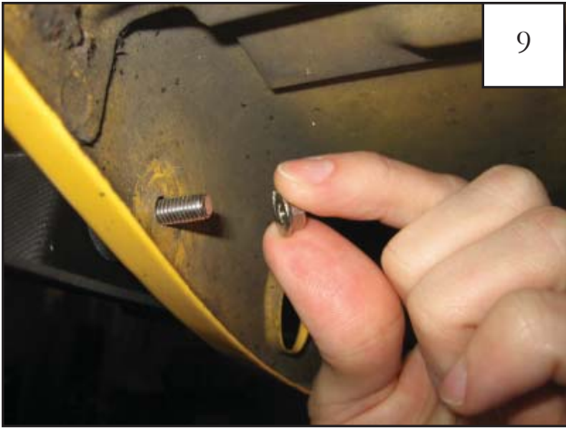
Step 2 Attach flange nuts to the threads on the M5-.8 machine screws and hand tighten.
