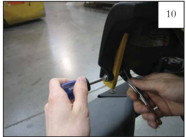
Step 3 Fully tighten flange nuts using a 5/16" socket and wrench and use a # 2 Phillips bit for the M5-.8 machine screws.
