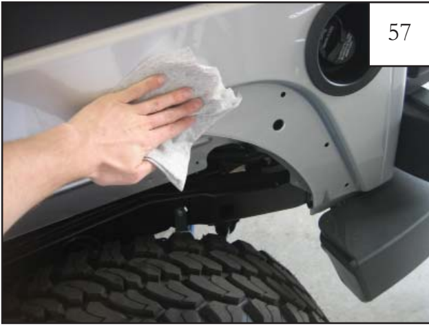
Thoroughly clean the exposed metal fender with a damp cloth then dry.
