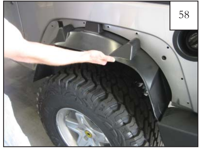
Hold the splash shield in place using supplied 1/4" Panel Retainers through factory holes halfway. Do not fully install Retainers, leave them half out. They are only used to hold splash shield in place for marking. See step 76 for locations.
