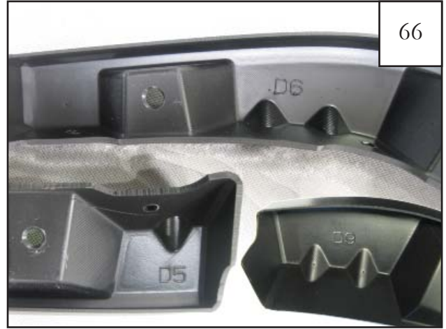
Locate the flat flare rear inner pieces. The driver side rear inner pieces are marked D5, D6 & D9. The passenger side front inner pieces are marked P5, P6 & P9.
