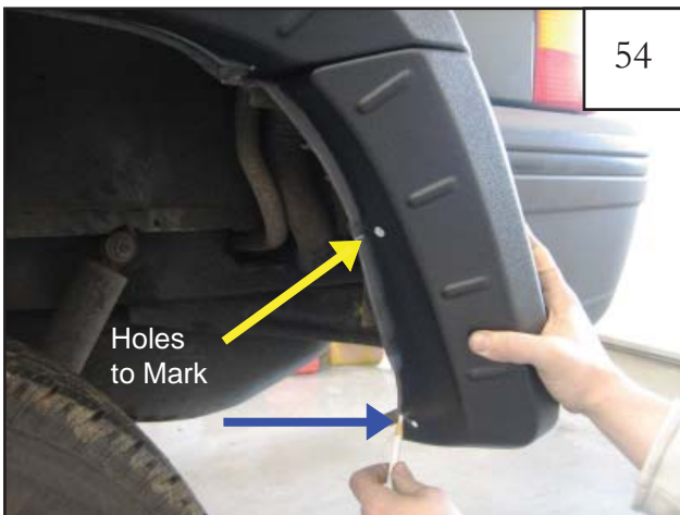
Hold the flare and bumper piece to the vehicle so that the bumper piece barely overlaps the cut bumper and mark the locations of the lowest hole and second highest hole on the bumper. Hole locations are white in picture for visibility. NOTE: See step 46 about gapping between bumper and bumper piece.
