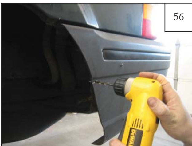
Using a 3/16" drill bit, drill the two marks made in step 55.
