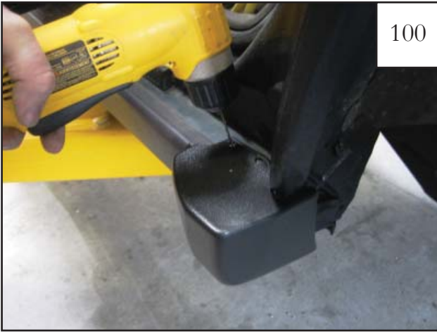
Drill marked holes with 3/32" drill bit.
