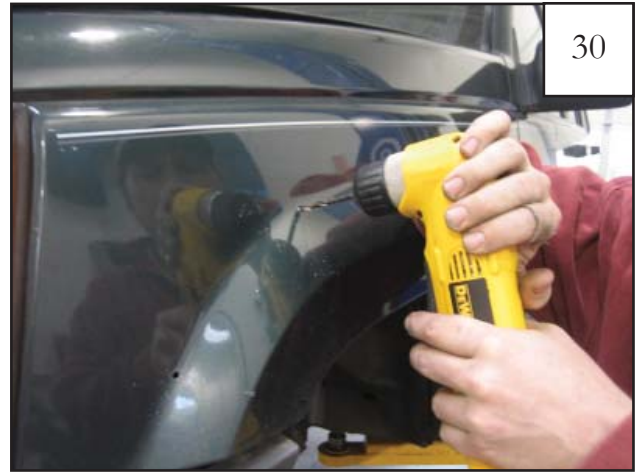
Drill holes in fender at marks with a 3/16" drill bit.
