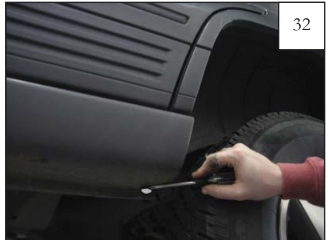
Remove christmas tree fastener from bottom of rocker panel near rear wheel well. Fastener is white in picture for visibility.
