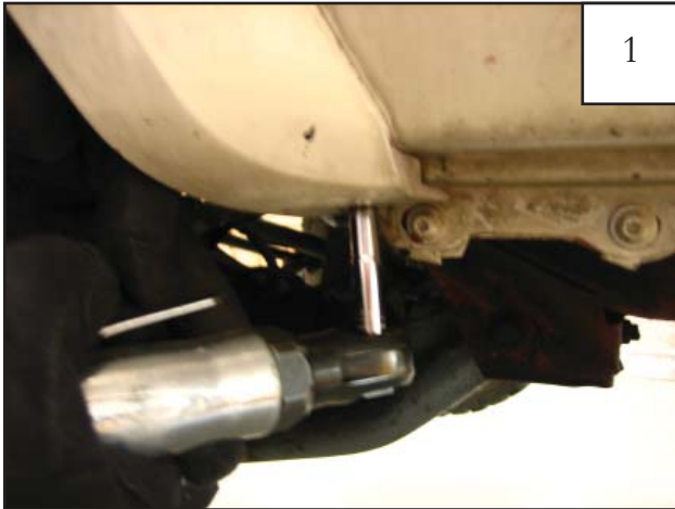
Remove the front factory flare starting with the lower rear factory fastener, using a 7mm socket.
