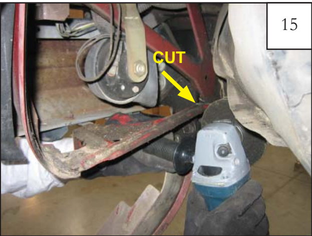
Carefully cut lower sheet metal strut attached to fender.
