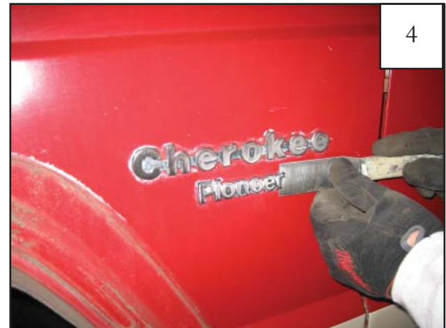
Apply adhesive remover to the Cherokee emblem for ease of removal. Using a putty knife, carefully remove the Cherokee emblem, taking caution not to scratch the paint.
