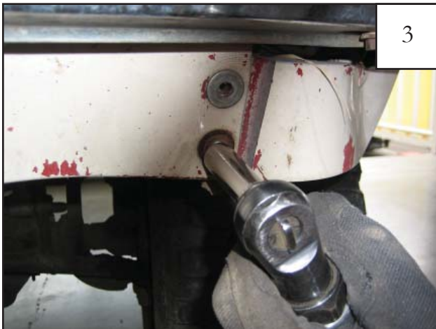
Using a 10mm socket, remove two factory fasteners underneath bumper on either side. Remove fascia piece
