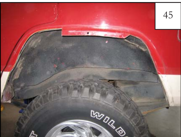
The fender should look like this. Some additional grinding may be needed. Optional: use caulking to seal all cut edges and seams.
