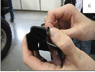
Make sure gimp and inner flare are clean. Peel 2" of liner from gimp (pin shape). Carefully position gimp as uniformly as possible along radius as shown, peeling liner as you go. Gimp can be repositioned as needed. NOTE: It is better for gimp to be slightly below radius rather than above.
