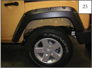
Ensure fit, and tighten all screws
