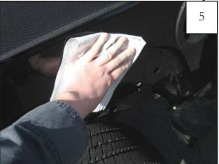
Clean fender area thoroughly with a soft clean cloth and isopropyl alcohol.
