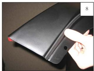
After gimp is properly placed, press to adhere properly and cut ends flush with ends of inner flare.
