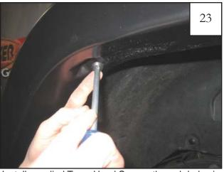
Install supplied Truss Head Screws through holes in wheel well and into #14 U-Clips installed in Step 15 (6 places).
