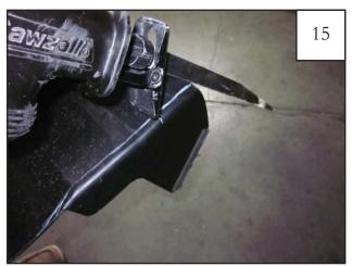
On front end of splash sheild using a grease pencil and mark in 1/2" from the radius of splash sheild and drawn a line till flush with outside edge of shield. Using a sawsall cut off section of splash sheild where indicated.
