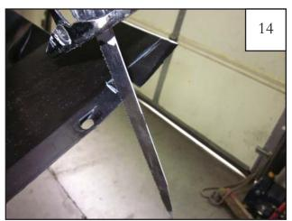
On rear end of splash sheild using a grease pencil, measure in from last hole 1-1/4" and make a line from the edge of shield to style line. Then create a line from the style line out to the end of the splash sheild as shown. Using sawsall to cut off section marked.
