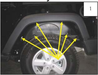
Using a pry tool, pliers, or flat head screwdriver, remove the six plastic fasteners from inside of splash sheild.
