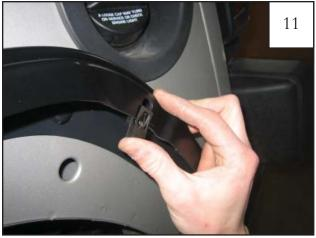
Install supplied "U" Nuts, with the thread side in, over holes in Inner Flare Piece (8 places).
