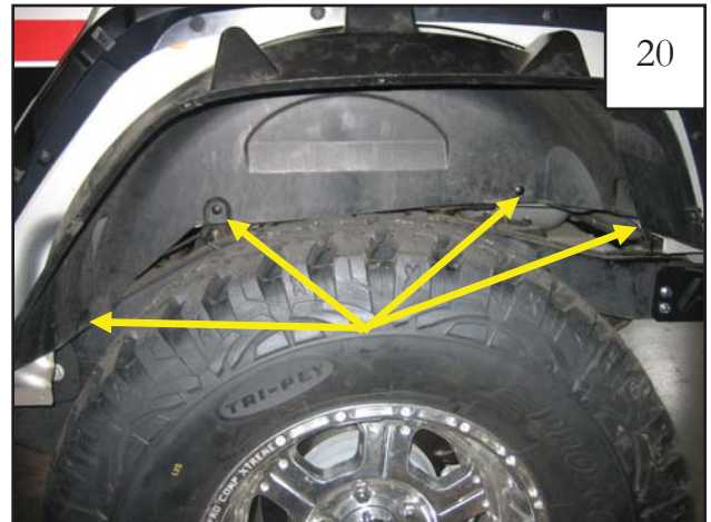
Install four supplied Plastic Phillips Head Tuflocs through splash shield and into vehicle body as shown.
